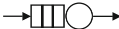
Fig. 2.24. The symbolic representation of a FIFO queueing server used throughout this book
