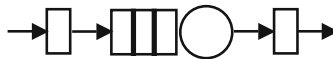
Fig. 2.23. Schematic representation of a customer or request arriving (from the left) into a line of customers waiting to be served. A customer that has received service is shown departing the server to the right
